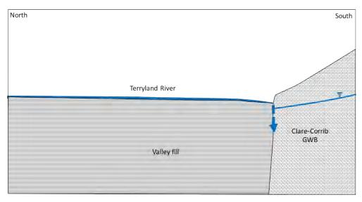
Plate 11 Schematic north south Cross-section through Terryland River showing the Operation of the Estavelles at Pollavurleen West and East during Low Groundwater Levels
