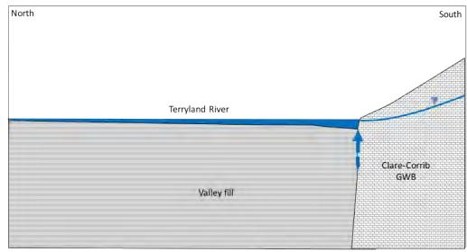
Plate 10 Schematic north south Cross-section through Terryland River showing the Operation of the Estavelles at Pollavurleen West and East during High Groundwater Levels
