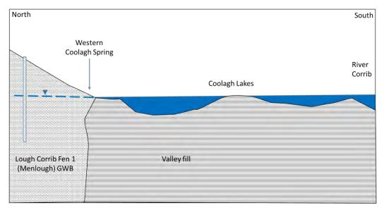
Plate 4 Schematic north south cross-section through Coolagh Lakes (groundwater low)
