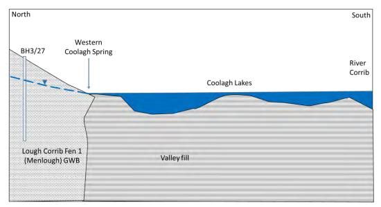
Plate 3 Schematic north south Cross-section through Coolagh Lakes (Groundwater High)
