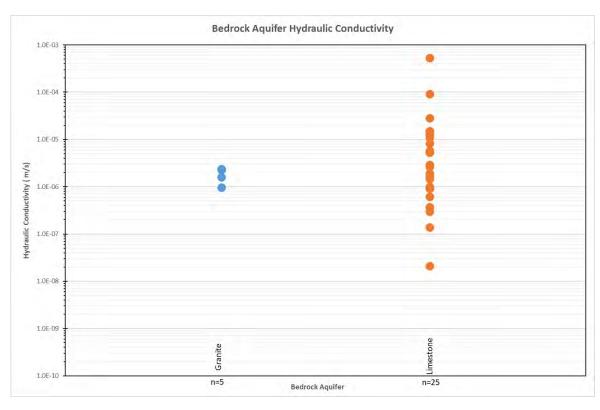
Plate 12 Distribution of Calculated Hydraulic Conductivity
