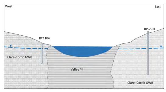
Plate 8 Schematic east west Cross-section through Ballindooley Lough showing the Interaction of Groundwater with the Lake during Low Groundwater Levels
